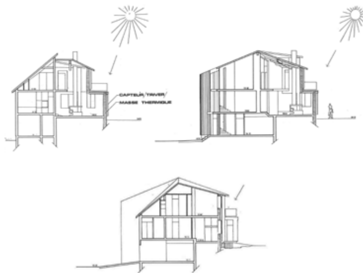
FIGURE 9 Three solar apartments in Odeillo, France. Sections with the dark Trombe Wall on two levels. (Architecture d'Aujourd'hui, 5/1973)
