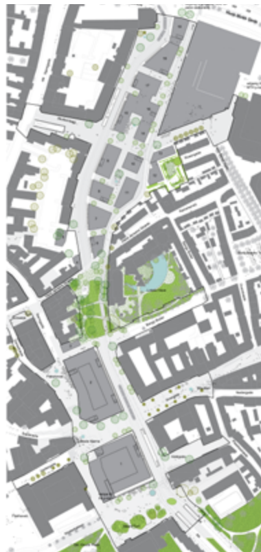
FIGURE 19 Plan showing the planned conditions at Thomas B. Thrige Street, with the new urban blocks, more narrow streets, and urban spaces.
