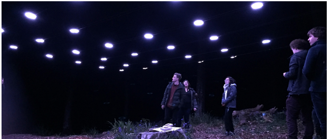
FIGURE 12 'Data-Space' – field of nodes containing infra-red sensors and LEDs, tracking human activities and communicating intelligent signals.
