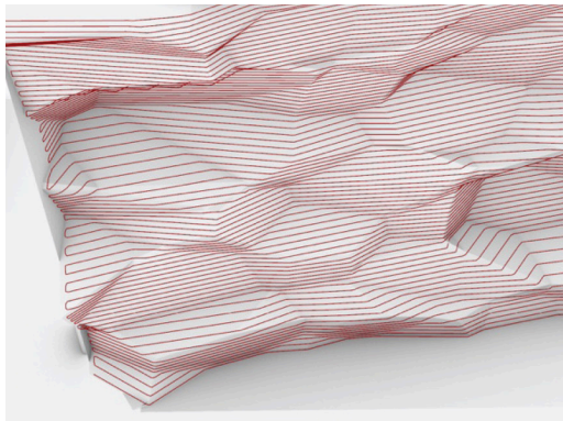
FIGURE 4 Robotic path optimization for subtractive D2RP
