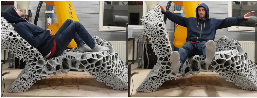
FIGURE 2 Chaise longue shape change from lying down (left) to sitting (right) obtained by tuning the stiffness through variable material deposition
