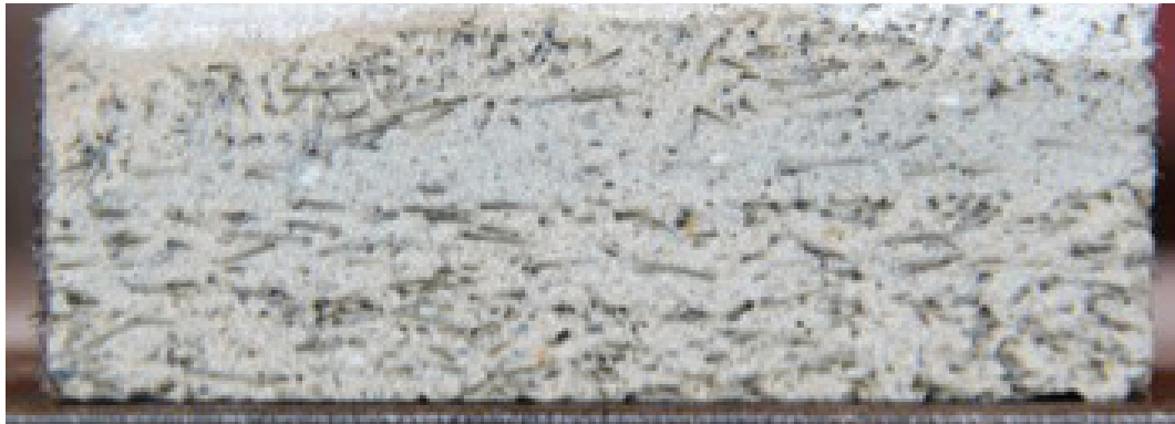
FIGURE 1 Parallel section of 3D printed concrete element, containing 6 mm steel fiber. (source: Raedts, W., MSc graduation, TU/e, 2017).
