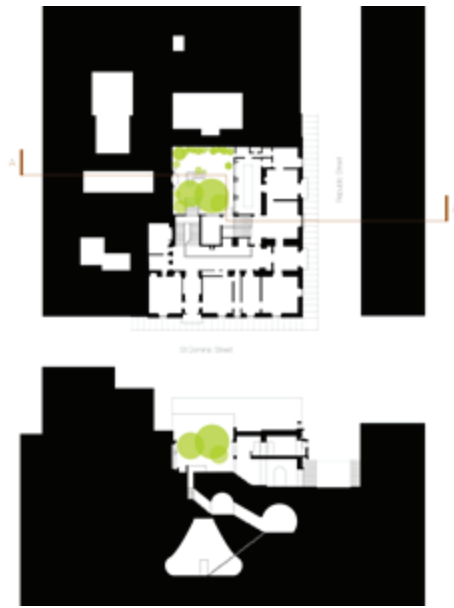
FIGURE 6 Contemporary plan and section of the Casa Rocca Piccola. The garden is caught between the levels of the house as the topography of the city falls down to the sea. The three carved cisterns below the garden are indicated.
