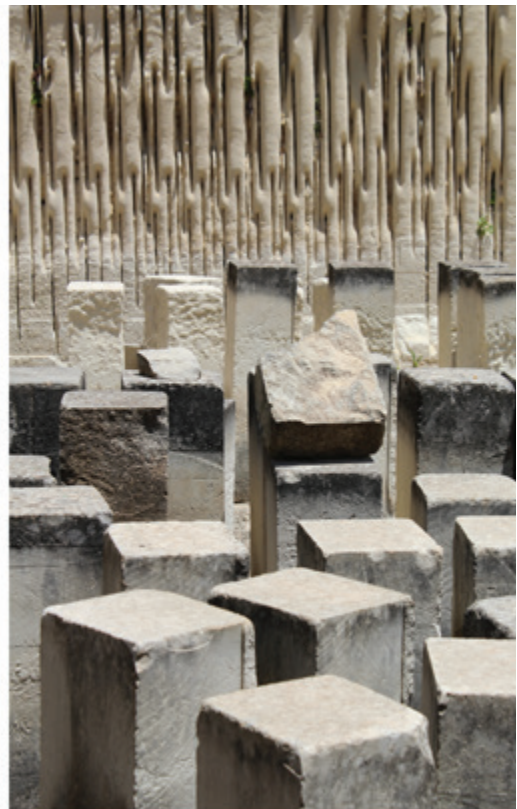
FIGURE 8 Franka limestone, the fourth layer of the island's geologic structure, being cut from the Siggiewi quarry. Franka is the primary material utilised in the construction of Valletta.
