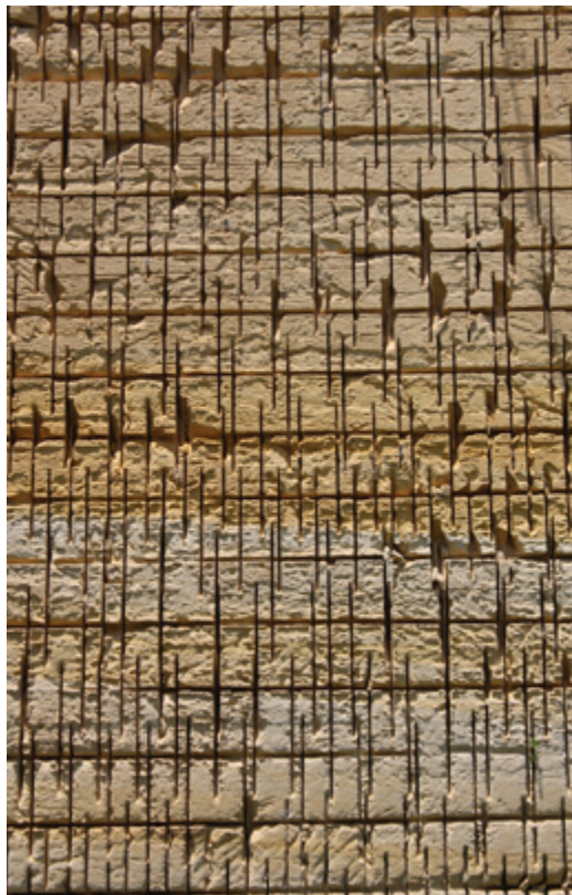
FIGURE 8 Franka limestone, the fourth layer of the island's geologic structure, being cut from the Siggiewi quarry. Franka is the primary material utilised in the construction of Valletta.
