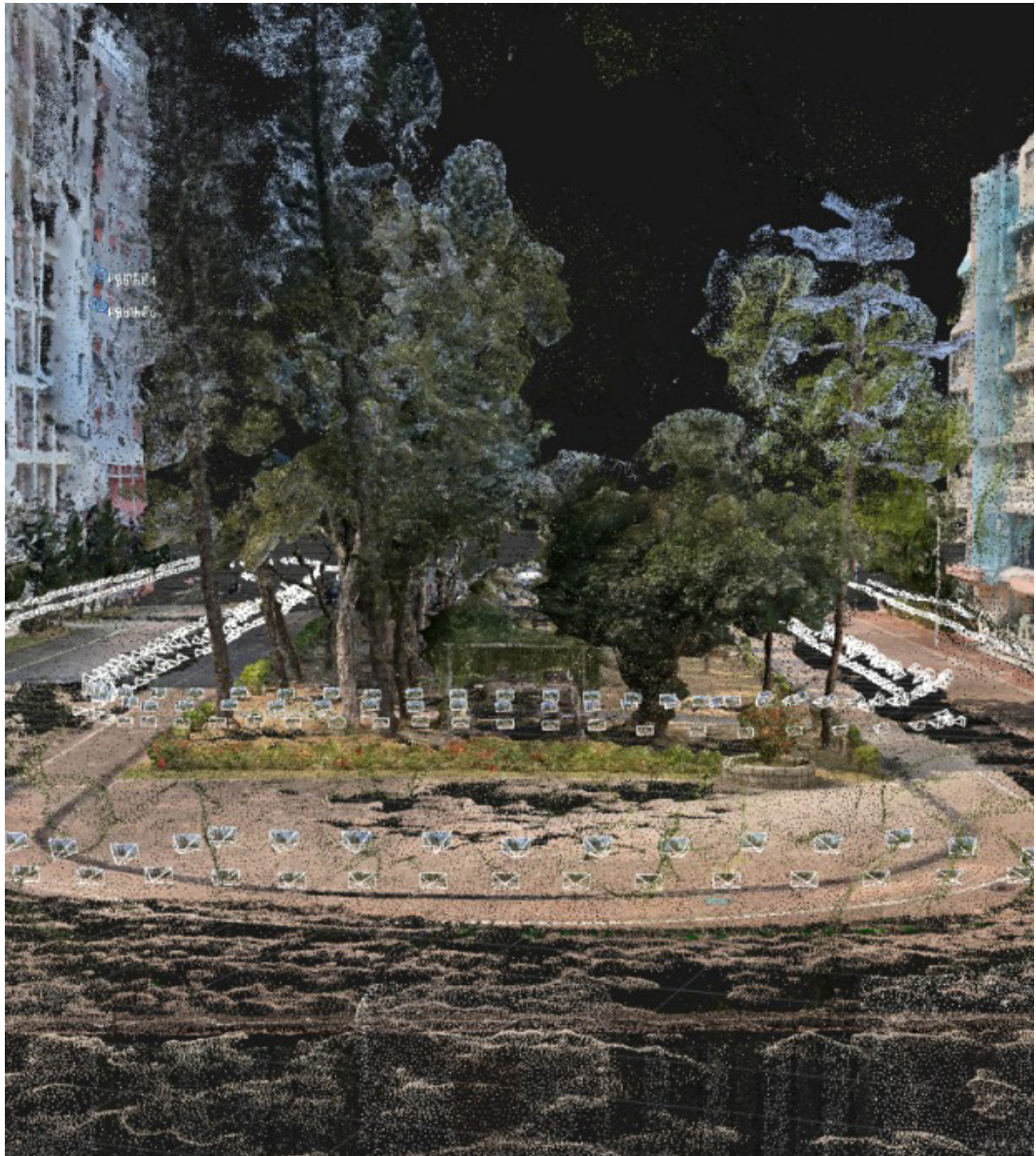
FIGURE 3 Point cloud model constructed with RealityCapture photogrammetry software, based on terrestrial photo datasets
