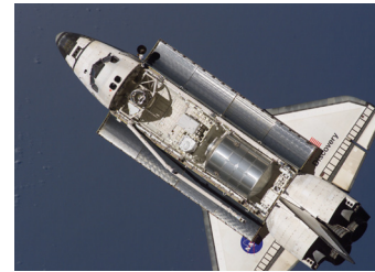
FIGURE 5 The space shuttle Discovery with its payload bay doors open. A module is resting inside the payload bay. (NASA)
