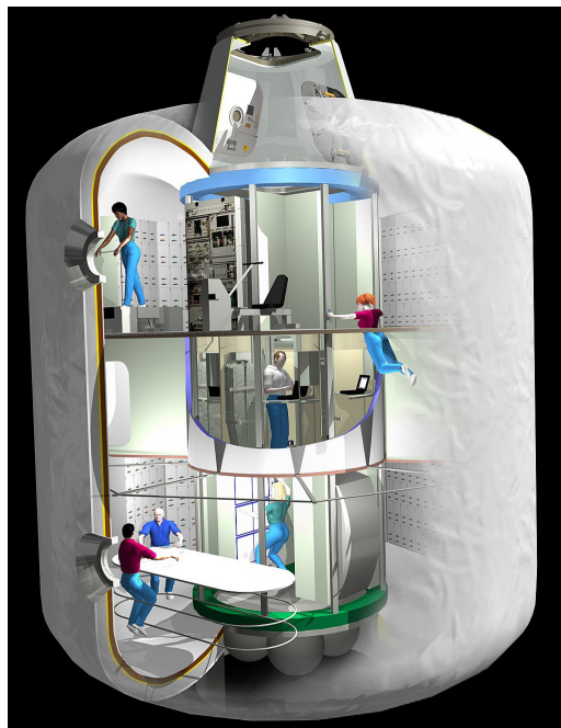
FIGURE 18 Cutaway of the Transhab Module. The inner core is protected by a so-called radiation shield water tank. (NASA)
