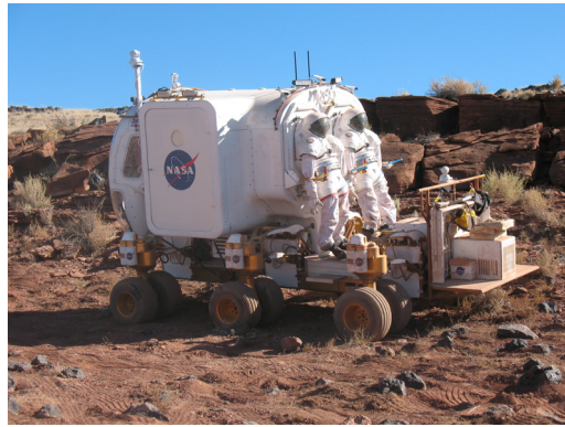
FIGURE 23 This is one prototype version for NASA's Lunar Electric Rover. This small pressurized rover is about the size of a pickup truck (with 12 wheels) and can house two astronauts for up to 14 days with sleeping and sanitary facilities. It is designed to require little or no maintenance, be able to travel thousands of miles climbing over rocks and up 40 degree slopes during its ten-year life exploring the harsh surface of the moon. Two spacesuits are attached to the rover suitlock. (NASA/Regan Geeseman)
