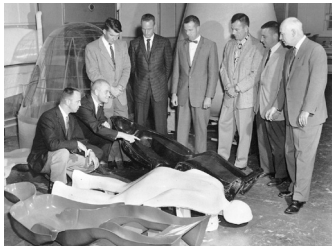
FIGURE 3 Mercury 7 astronauts examine their ‘couches’. Each astronaut’s couch was moulded to fit his body to help withstand the G-loads of the launch.1959 (NASA)
