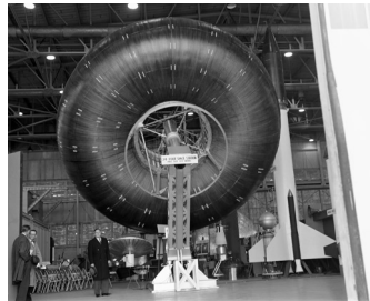
FIGURE 12 This 1961 prototype of an inflatable space station concept with a solar power system collector was 7.3 m (24 feet) in diameter with an internal fabric bulkhead that could be separately pressurized in an emergency. (NASA)
