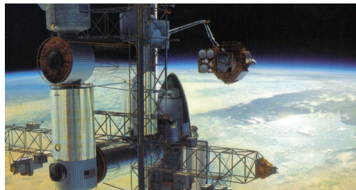
FIGURE 1 Early space station concept by Boeing in 1984. At that stage, it was required to have two ways to exit each module. The modules would be linked in a loop configuration. (Illustration by Paul Hudson)
