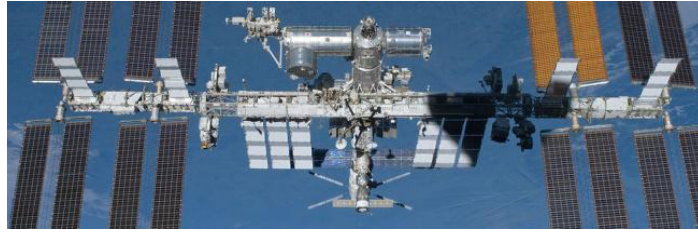
FIGURE 7 The International Space Station with its truss structure for the photovoltaic system, 2020 (NASA)
