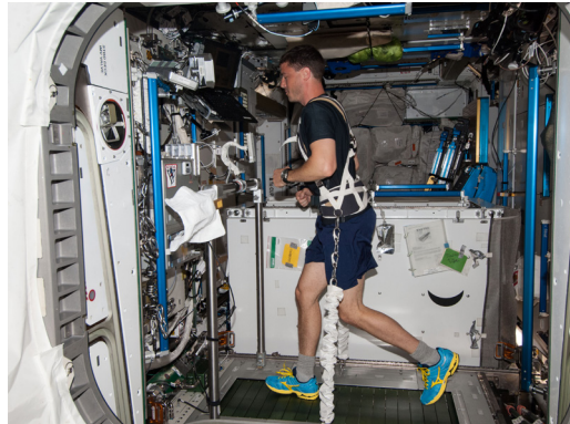
FIGURE 32 NASA astronaut Reid Wiseman, equipped with a bungee harness, exercises on the T2 treadmill. (NASA)
