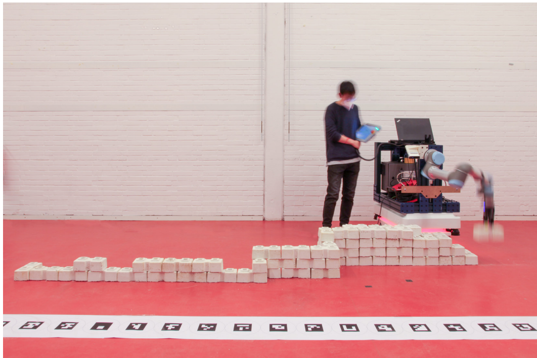
FIGURE 11 The wall assembled by MiRo with the QR code markers on a banner on the floor. Authors, 2023.
