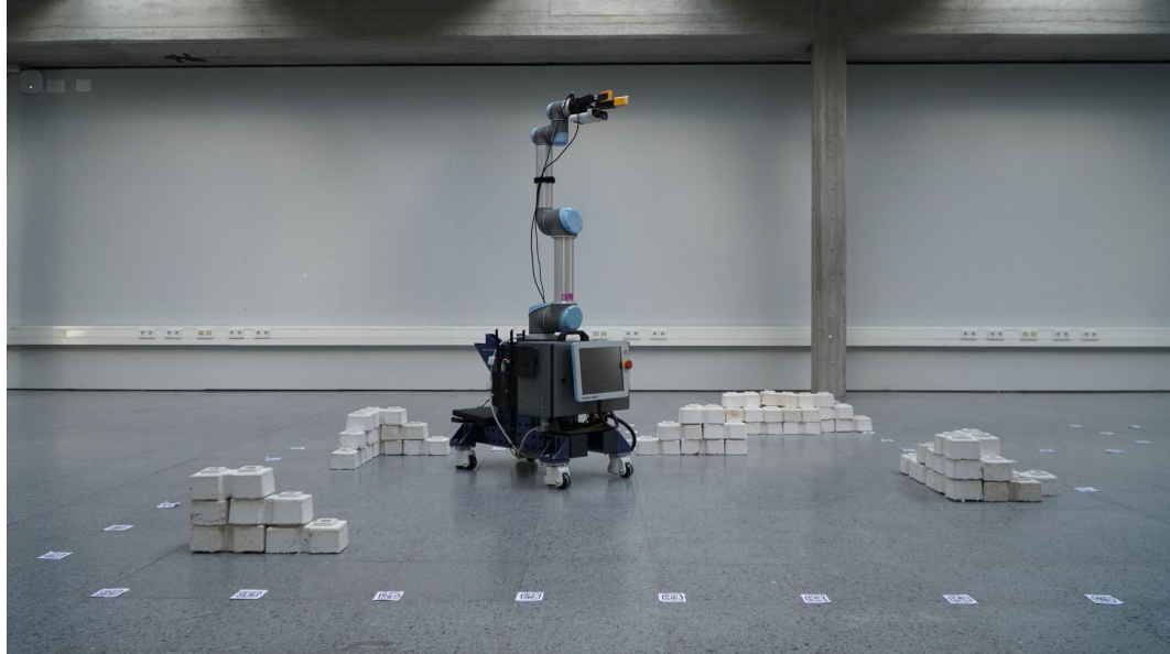
FIGURE 7 UR5 with Kinect camera on wheels, reactIVision markers on the tile grid, and the custom bricks placed in the corners of an unbuilt wall. Authors, 2023.
