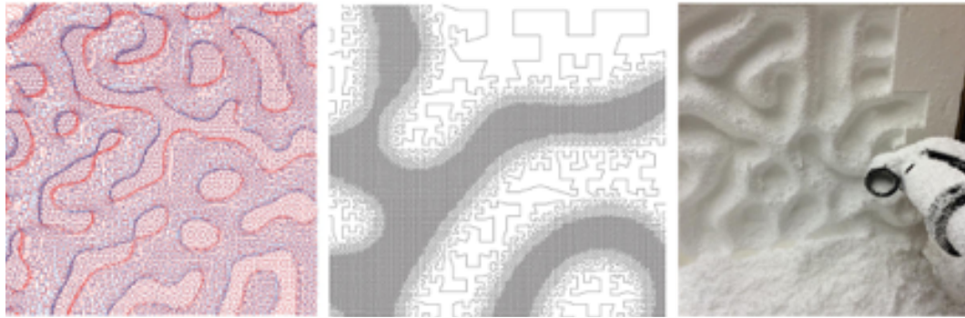
FIGURE 1 Recursive milling method: left - with homogenous resolution; middle - tool path with informed resolution based on material removal; right - prototyping.
