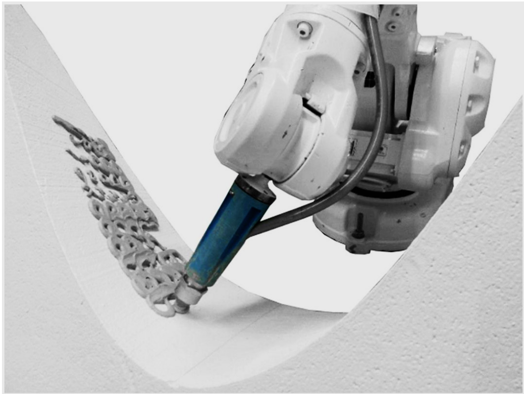
FIGURE 4 Scalable Porosity: Customised robotic set-up for 3D printing on ruled surfaces
