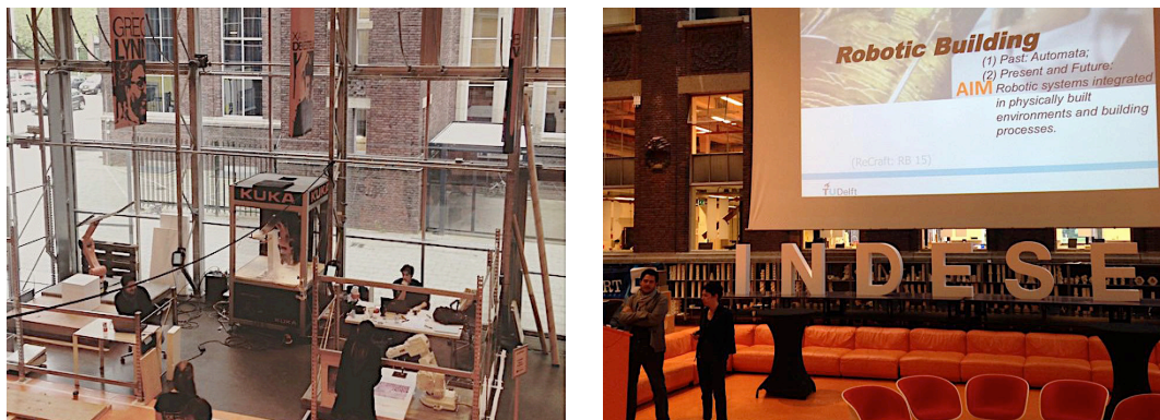
FIGURE 3 InDeSem: Deployable setup of three robots using several fabrication techniques (wire cutting, milling and drawing)
